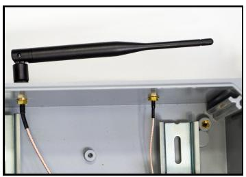
12) Cellular and WiFi antennas should be connected outside of the enclosure. If installed outdoors, ensure the seals are water-tight.
