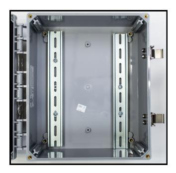
2) The two 13" pieces of DIN rail should already be mounted in the enclosure. Using a screwdriver, check to make sure they are tightly fastened.
