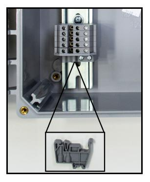
3) Take the 5 gray terminal block pieces and connect them to the DIN rail. Use the gray cover plate to cover one end. Add a terminal endstop to one side of the terminal block. Wait to fully tighten the screws on the endstop as you may need to adjust it later.
