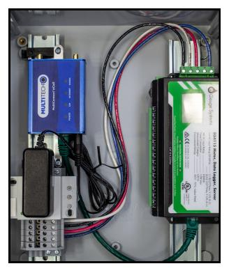
9) Cut lengths (approximately 7" long) from each section of colored wire. Use these to connect the five pin power plug on the eGauge to the terminal blocks. For U.S. 120/208V NEC color coding, the white wire should connect to the "N" terminal, black to "L1", red to "L2", and blue to "L3" (if applicable).
