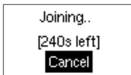
**WPS Setup** – connects the eGauge to a router using WPS push-button pairing. To perform WPS setup, consult your router’s manual. Generally this process requires holding a button labeled “WPS” on your router between 1 and several seconds, then initiating the “WPS Setup” function on the eGauge.
