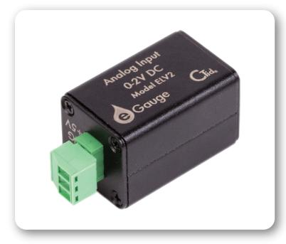
The eGauge 2V Analog Input Sensor allows EG4xxx meters to read 0 – 2V analog values or dry contact states from standard 2-wire dry contacts such as relays. The Analog Sensor requires the eGauge Sensor Hub (ESH044). Wiring diagrams for the Sensor Hub and compatible sensors can be found on the following page.
