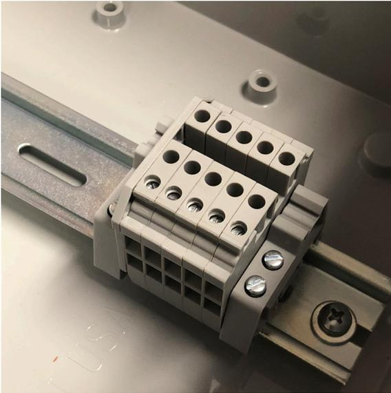
3) Take the 5 gray terminal block pieces and connect them to the DIN rail. Use the gray end plate to cover the exposed end. Connect a terminal end stopper to each side of the terminal block. Wait to use the screws to secure the block as you may need to adjust it later.
