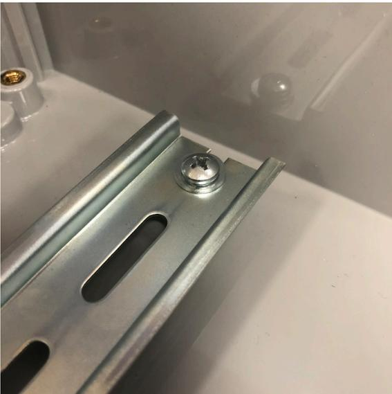
2) The two 13" pieces of DIN rail should already be mounted in the enclosure. With a Phillips head screwdriver, check to make sure they are tightly screwed in place.
