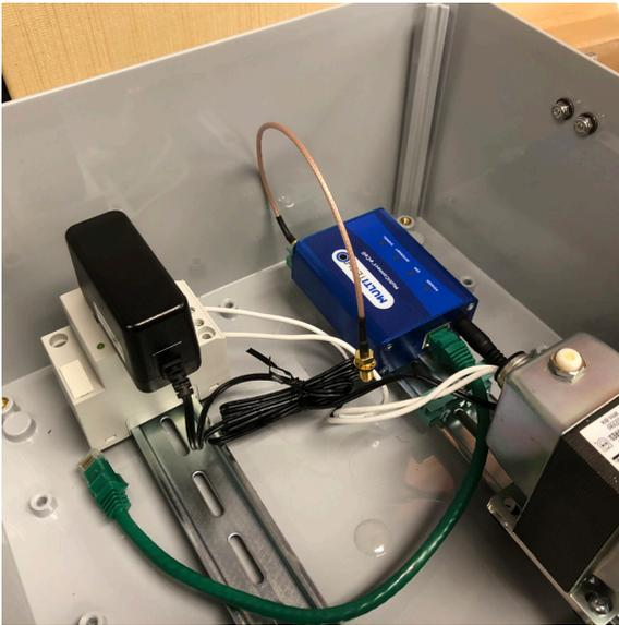
8) Attach the cell router or other accessory. Cell modems use a DIN clip to attach to the rail.
