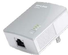
The HomePlug AV200 power-line adapter uses your home's existing electrical wiring to create a direct connection between your eGauge meter and a home network. This connection requires no additional wiring and you can simply plug the adapter into existing power sockets to instantly establish a networking infrastructure.
