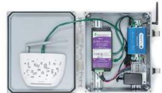
The Powered Enclosure Kit is designed for installation of the eGauge in combination with one of several communication protocol devices. The kit comes with components that complement the eGauge main unit, decreasing installation time and reducing complexity. Included: (1) NEMA4 polycarbonate enclosure, (2) DIN rail pieces, (1) Power distribution block, (1) 120VAC receptacle, (1) Wire set, (1) Mounting Kit. The PEK-277 also includes one PT-50VA. *Shipped Unassembled*
