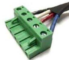
The Power Whip is an installation component used to connect the eGauge meter to a breaker panel. Each Power Whip includes a 5-pin Power Plug and four 8' lengths of THHN #12 stranded copper wire with NEC compliant colors for L1, L2, N, and L3.
