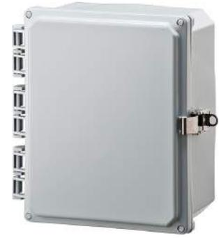
Integra polycarbonate enclosure, hinged and lockable lid, DIN rail and mounting kit included. Key Specifications: Temperature Range = -40 to 265 °F, Flame Rating = UL, 5VA. (Test Spec. UL-94), Outdoor UV Exposure = F1. (Test Spec UL), UL-50/c-UL Type 4X Listed (file #E207562) IP 66 .
