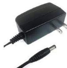
A standard power supply to convert 100-240VAC @ 0.5A (50/60Hz) to +12VDC @ 1A. Called a “switching adapter”, this product has a 2-prong US style plug that connects to a wall outlet and a barrel jack for connecting to other hardware. It is UL listed and FCC compliant, with an efficiency level of V.
