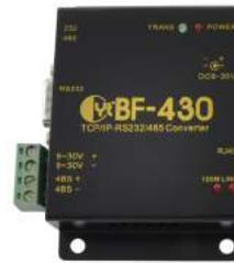
The RS485 to Ethernet Converter is a universal serial device server that enables users to connect Modbus RS485 sensors to the eGauge using a local area network. The BF430 requires a power supply (EA1001, page 8) or a direct +/- 9-30VDC connection for power.
