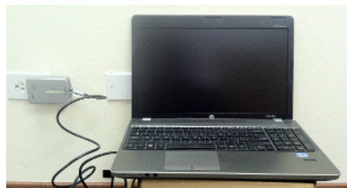
Figure 6.2: Laptop connected to a HomePlug adapter
